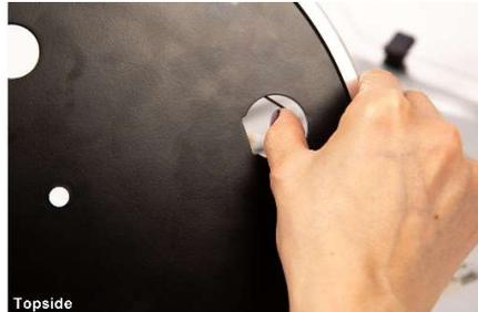
6. Gently lower the platter onto the central spindle of the base unit, ensuring that the elastic band is stretched over the drive shaft.
